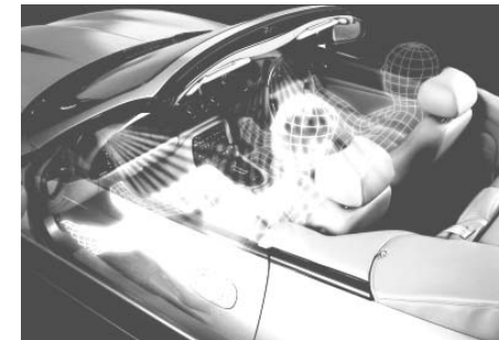
Fig. 13-6: Occupant classification for optimal airbag activation [WES02]
