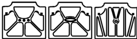
Fig. 11-9: Passive optimisation of the bonnet structure
