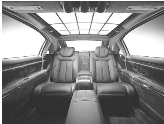
Fig. 6-23: Electrochromic panorama roof in the Maybach 62
