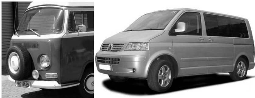
Fig. 6-17: Rubber profile glazing at the VW Type 2, year of construction 1967 (left) and bonded windscreen and rear window at the actual Multivan (right)
