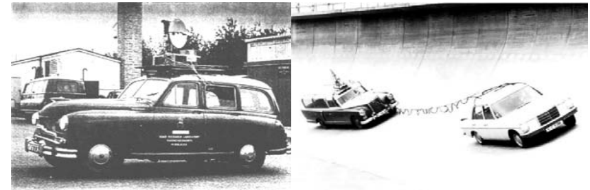
Fig. 8-12: First driver assistance systems to take over driving tasks; left: vehicle with a radar sensor; right: vehicles with vehicle-to-vehicle communication
