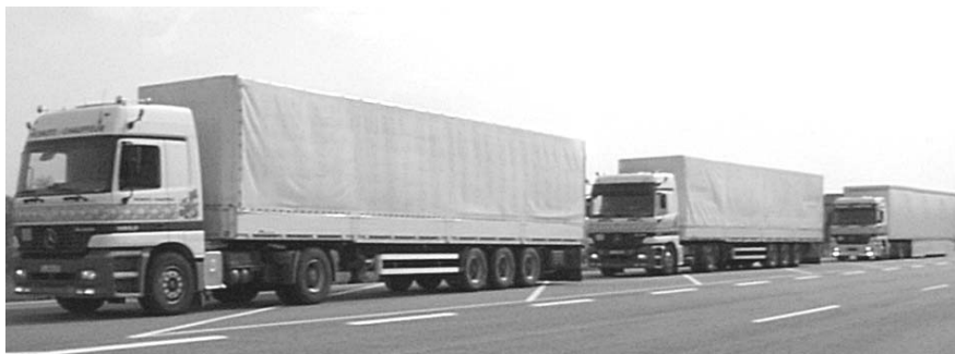
Fig. 8-32: electronic tow bar in the PROMOTE CHAUFFEUR 2 project [BON03]
